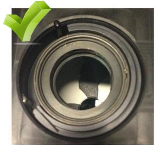
The Iris lever and the Silver pin are on the same side, it will be impossible to lock the Iris back
