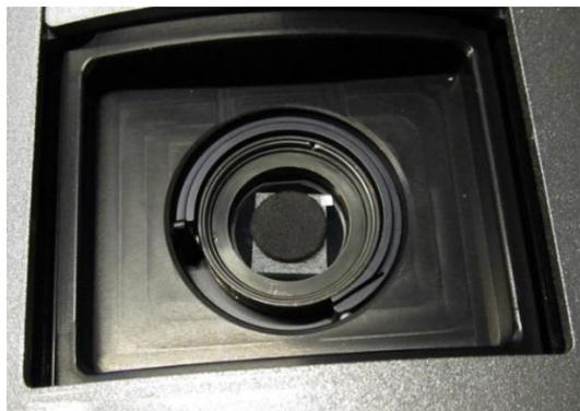
2.1.2. The sponge is placed on top of a rice paper on the stage window. The rice paper prevents the sponge particles reaching the stage. When closing the centering Iris on the sponge, the sponge is pressed preventing the window to move freely.
